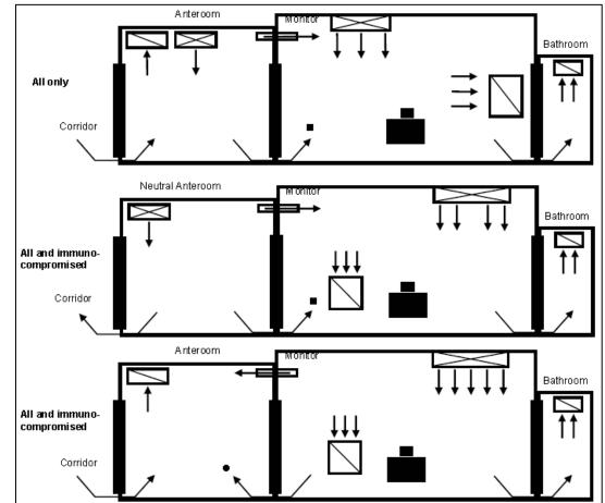
Figure 4. Example of airborne infection isolation (AII) room with anteroom and neutral anteroom\* + \$
